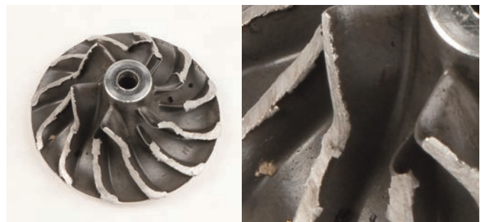
Compressor wheel rub
