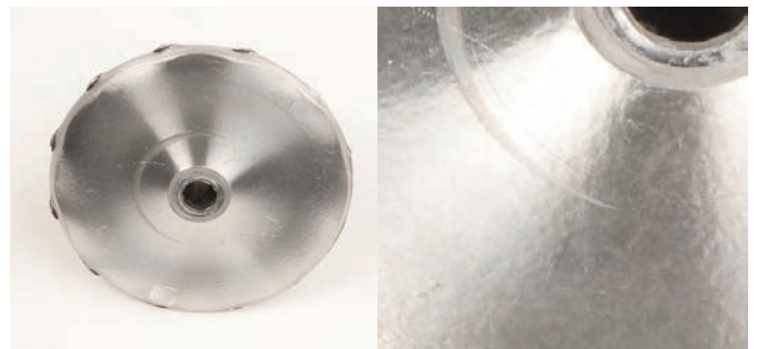
The 'orange peel' effect on compressor wheels
